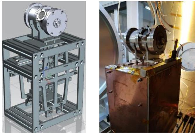
Figure 6. a) Schematic of the BUSTLab MET on the thrust stand, b) MET on thrust stand before tests
