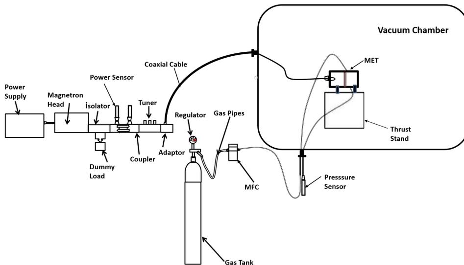
Figure 2. Schematic view of the experimental setup
