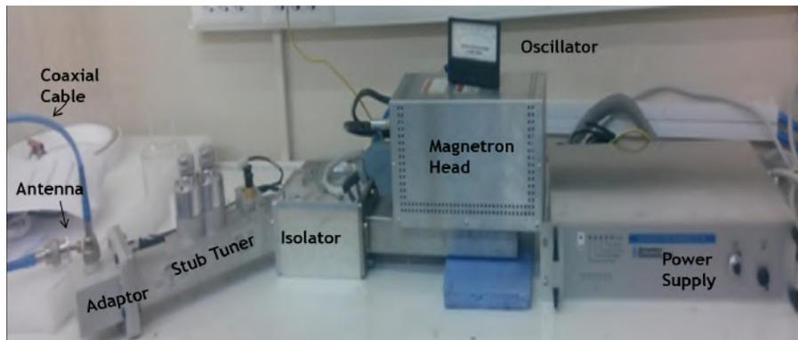
**Figure 3. Picture of microwave power generation system.**
