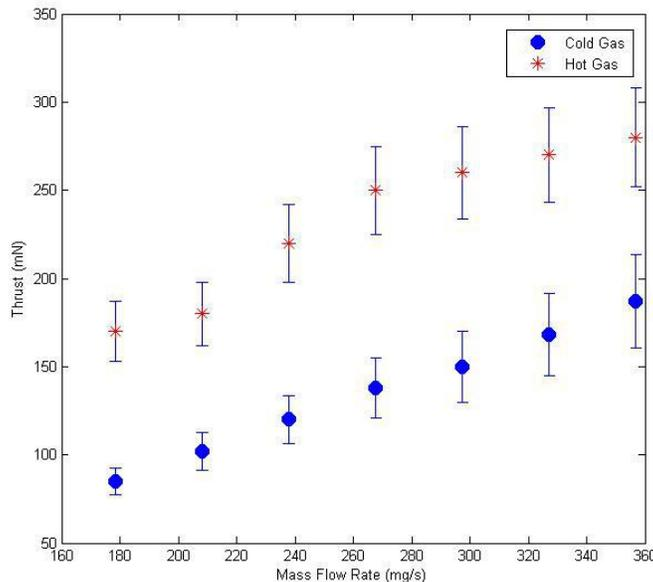
**Figure 8. Thrust vs. mass flow rate for the cold gas case and for the case with 200 W of power delivered**
